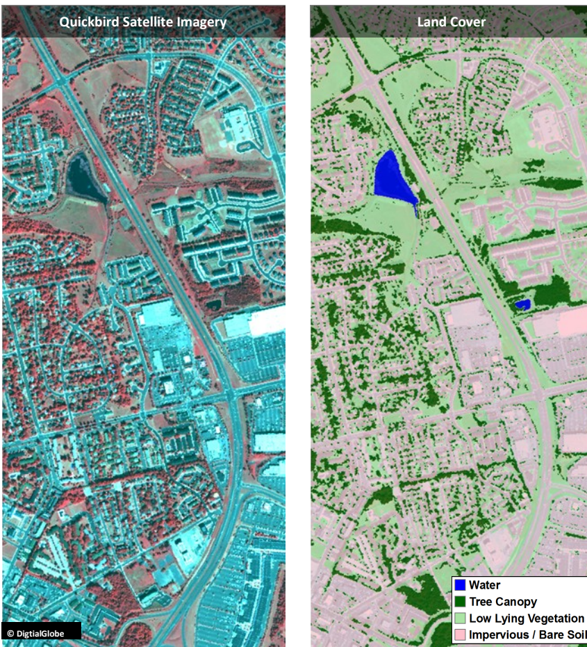
Figure 1: Land cover mapped from satellite imagery. The satellite imagery used for this project was acquired by the Quickbird satellite in October 2007 at a resolution of 60 centimeters.
