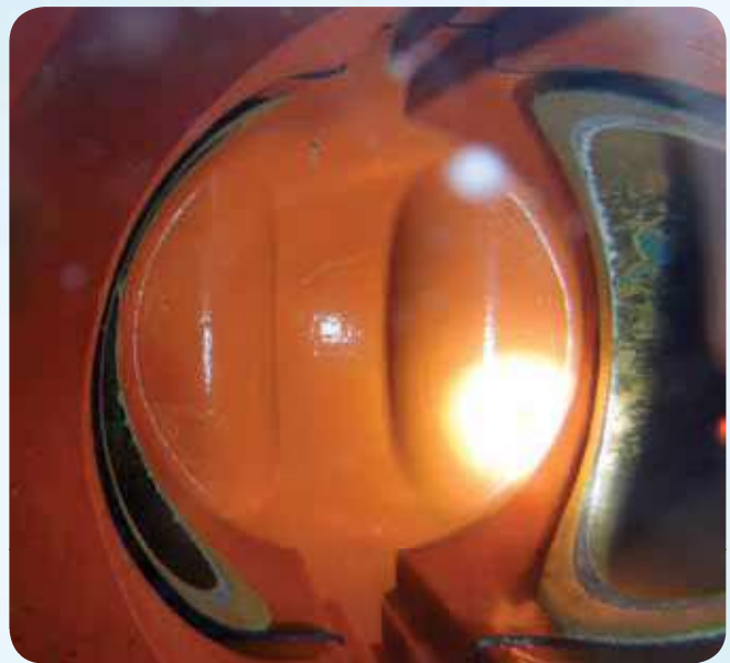
An under-pressure look of clean valve seat.
