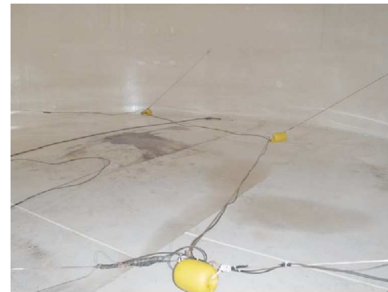
FLOATING RING CATHODIC PROTECTION SYSTEM NO SCALE
