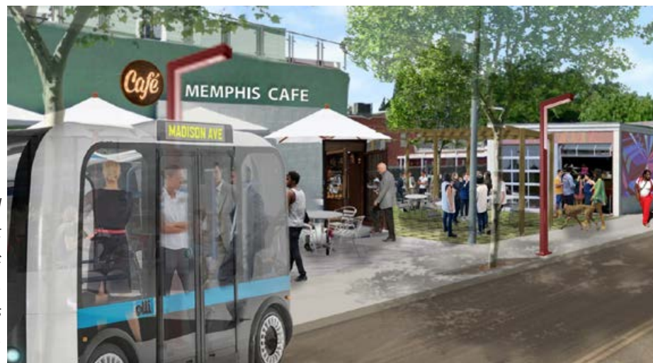
Example of a slow-speed automated shuttle that can operate in mixed traffic and provide inexpensive, high frequency connections along fixed routes.
