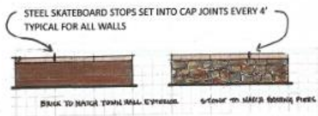
Typical Wall Elevations
